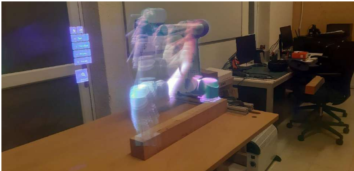
Figure 18. Geometry representing the robot's full range of motion at a given instruction, displayed through the mixed reality headset.
