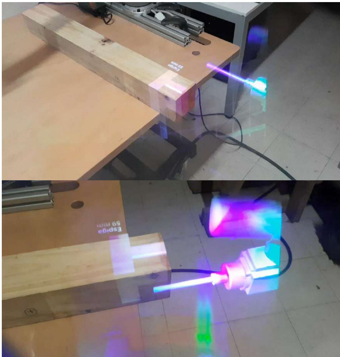
Figure 20. Tenon milling preview through MR-HMD. Displacement of visual guidance.
