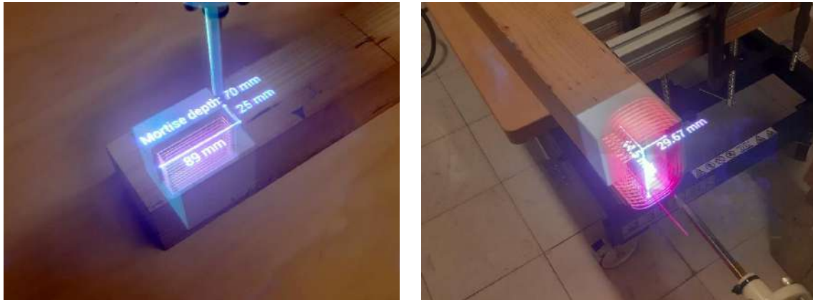
Figure 21. Display of different positioning results for visual guides, as viewed through the MR-HMD, HoloLens 2.
