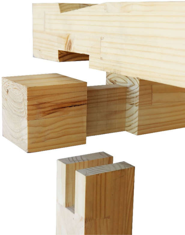
Fig. 3 A knot composed of T-bridle jointed post and top plate with notched tie beam and oblique mortise on top
