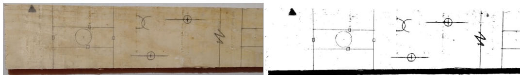
FIGURE 11. Effective use of the k -means algorithm for color-based segmentation of hand-drawn carpentry drawings. The original image is on the left, and the segmented one is on the right.
